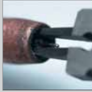
Spatter removal from in and outside the nozzle.
