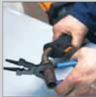
Nozzle removal and installation.
