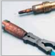
Spatter removal from the nozzle end.
